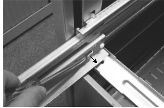
If you experience problems fitting the back of the drawer into the slots on the suspension slide inner members, you can open the slots slightly with a plain slot screwdriver.
