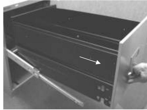
Open the drawer to full extension, and raise the front clear of the suspension slide inner members.
