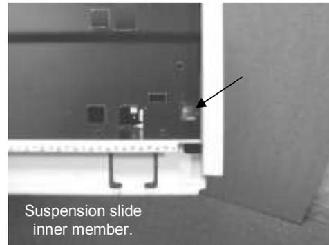
Once both tags are clear of the suspension slide inner member, the front of the drawer can be raised removed.
