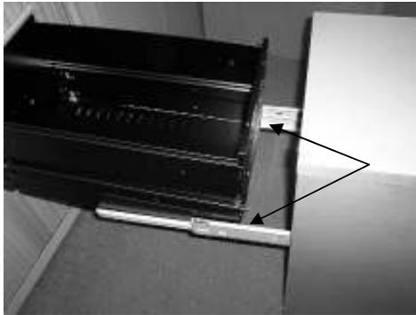
When fitting, rest the rear of the drawer onto the suspension slides inner members.
