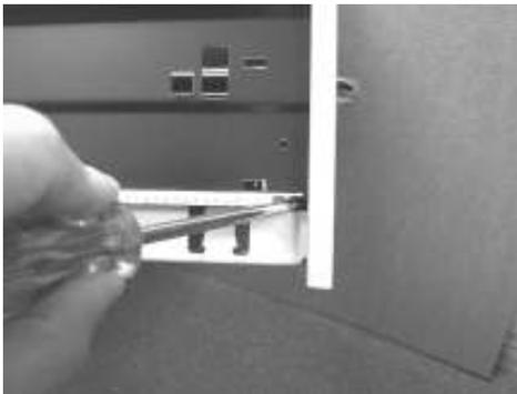
Each fold over tag can be pushed back flush with the drawer body using a plain slot screwdriver.
