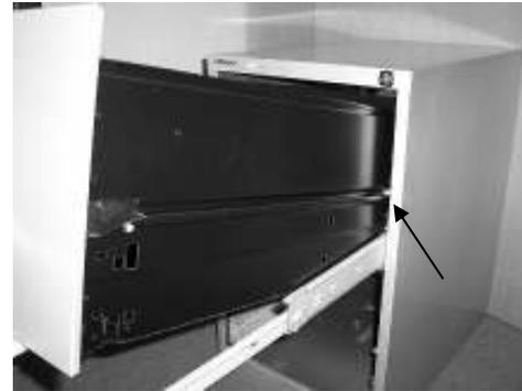
Slide the drawer backwards into the cabinet, tilting the front up, to locate the right side edge of the drawer underneath the plastic locking bar tag.
