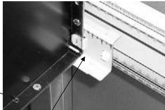
The suspension slide inner members have a cut out slot for the rear of the drawer to fit into.
