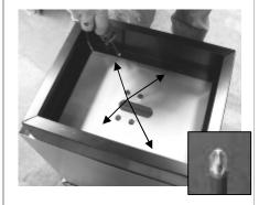
Tighten screws using a crosshead screwdriver
