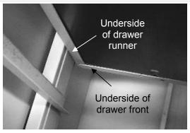
It is hard to remove a drawer which has been fitted handle first, this is because the return folds on the drawer front (top and bottom) prevent the drawer from fitting back out through the drawer runners (As above)
