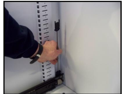
Insert an anti-tilt connector into the top rear of the existing runner ensuring both plastic connectors have the flat side facing the carcass.
