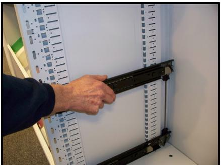
Ensure the bottom runner is extended and locate the next runner by inserting the anti tilt connector into the underneath of it & fix in place by first inserting the rear lugs then the front as before.
