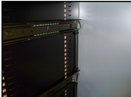
If more than one roll out fitment is required then the anti-tilt mechanism needs to be fitted to ensure only one can be rolled out at a time for safety. *The following photos are not of roll out fitments but the procedure is the same*
