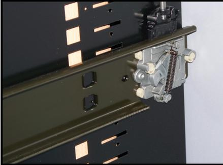
Locate the runners into the unit ensuring enough space from bottom for clearance of hanging files. To attach the runner locate the two rear lugs into the cutouts on the inner skin and push the runner towards the back of the unit.
