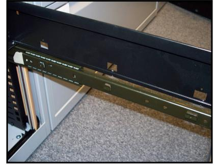
The roll out fitment will attach to the runner on 3 metal lugs on each runner. Extend the runners on both sides fully and locate the cutouts on the fitment onto the lugs on the runners.
