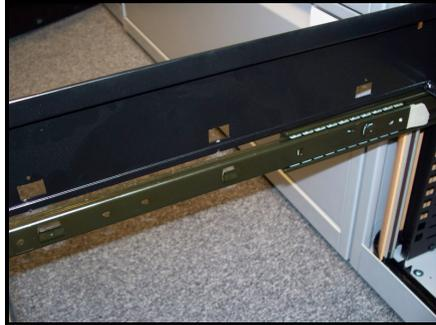
Extend the runner and locate the two front lugs into the corresponding cut outs at the front of the unit and push downwards firmly to fit into place. Repeat this with the runner on the opposite side
