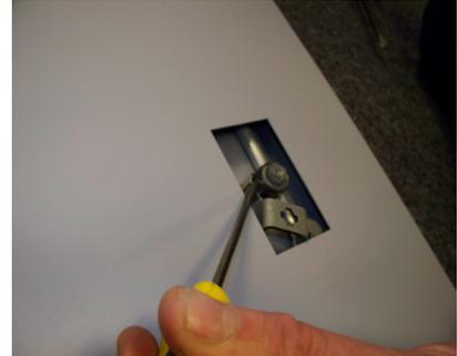
Using a flat head screwdriver unclip the spring clip which holds the lock in place. The lock can then be removed from the door completely.
