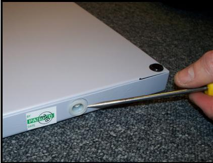
If the locking bar has fallen inside the door you will need to retrieve it. Remove the plastic locking bar guide from either end of the cupboard door using a flat head screwdriver.
