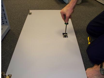
Remove the door from the cupboard and lay down on its front. Using an appropriate screwdriver remove the screw in the back of the lock and move the locking bar away from the lock
