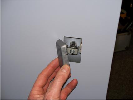
If the locking bar has fallen inside the cupboard, to retrieve it firstly you would need to remove the lock from the door. Remove the protective cover to reveal the lock mechanism
