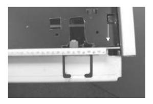
Close up view of the location slots on the front of the left-hand suspension slide inner member.
