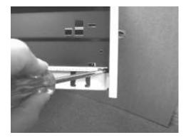
Each fold over tag can be pushed back flush with the drawer body using a plain slot screwdriver.
