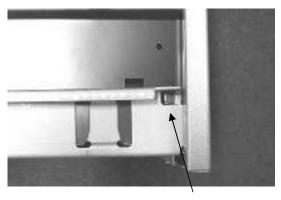
Push the drawer down fully into the location slots on the suspension slide inner members, to allow for the fold out securing tags to align correctly.
