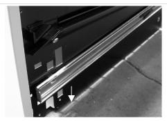
This will allow the drawer to be lifted upwards away from the slide front 'tag lancings'.
