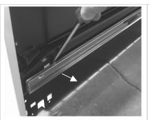
Use a slot headed screwdriver to lever the slide inner member away from the drawer, for the retaining pip.
