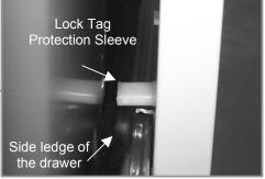
When fitting make sure the right hand side ledge of the drawer is located underneath the locking bar, lock pin. (This can be awkward)
