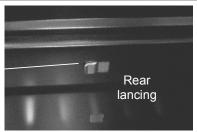
Place drawer centrally between the slides, (Supporting the weight of the drawer) locate one of the rear lancings into the rear slot on the drawer, then drop the front of the drawer into the front lancing on the same side, before repeating the procedure with the opposite side of the drawer.
